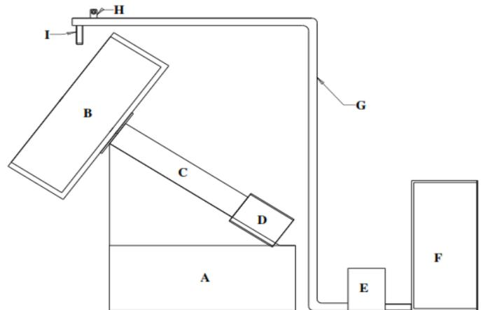
Figure 1: Schematic diagram of the granulating system: Pan (B) is connected to an electric motor with a variable gear (D) with shaft (C). Pan (B), Shaft (C) and gear electric motor (D) was supported by stand (A). A Solution of binder was pumped through pipe (G) with a surface pressure pump (I) from reservoir (F) and binding solution was sprayed on to the materials through nozzle (G) which was being regulated with valve (H).
