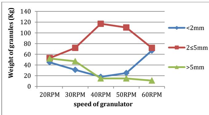
Fig.2. Effect of rotational speed on size distribution of granules formed.
